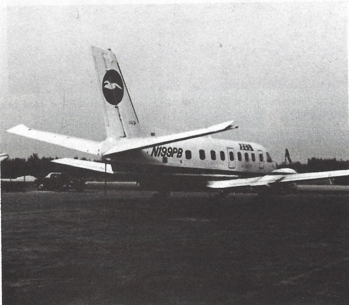
PBA's two newest Bandeirantes arrived from Brazil during December. The most notable exterior change is the dihedral in the horizontal stabilizer which is designed to eliminate vibration. Improved insulation and other interior improvements have brought comments from both pilots and passengers that the new Bandeirante is a smoother flying and better aircraft.
